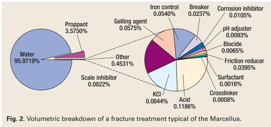
Fig. 2. Volumetric breakdown of a fracture treatment typical of the Marcellus.
